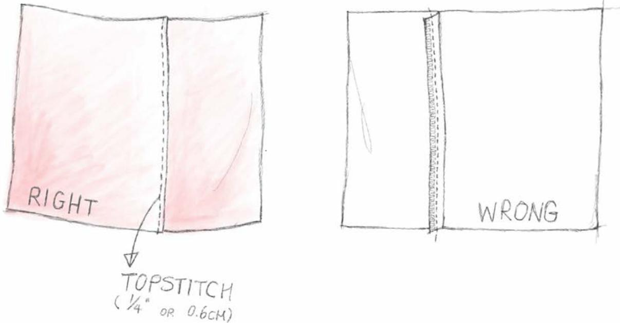
The purpose of top stitches are to add strength to the garment. Iron the seam allowance to the side. Straight stitch  $\frac{1}{8}$ " or 0.3cm, or  $\frac{1}{4}$ " or 0.6cm away from the original seam to sew the right side and seam allowance together.
