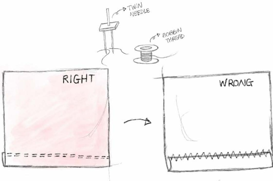
Twin needles are used in knit casual or sportswear for clean finishing without needing a double fold hemming method. The 2 top threads and 1 bobbin thread create parallel topstitch on the right side of the fabric and zigzag stitch on the wrong side of the fabric.
