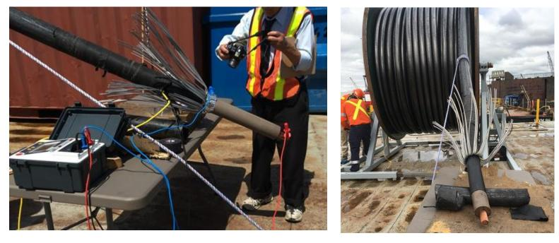
IR test using the guard probe ( blue wire) at the cable shield for better reading
