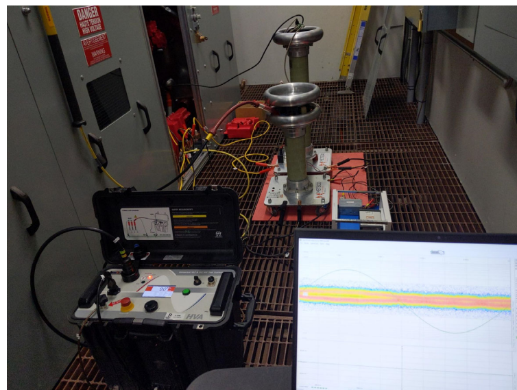
Figure 6. Simultaneous VLF Tan-Delta and PD Measurement Setup.
