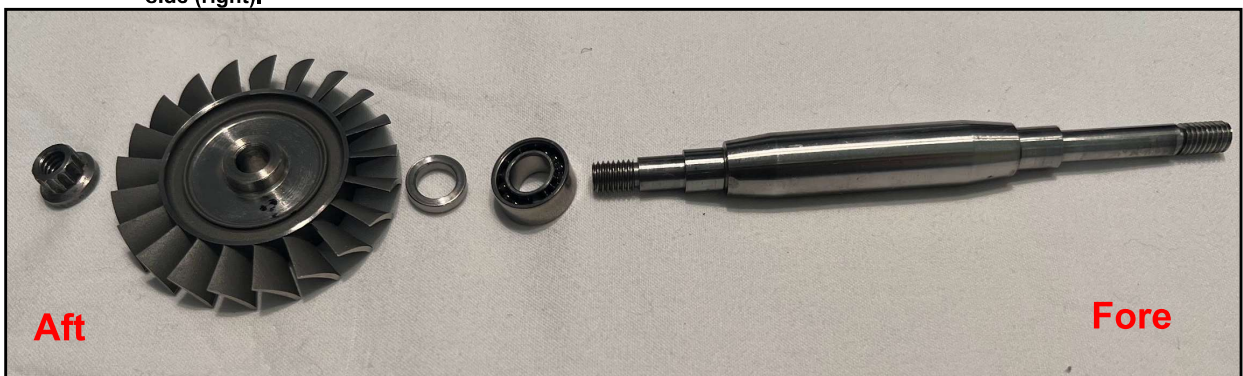
Figure 3: Image of bearings. Notice the slightly smaller gap where the ball bearings sit on the “pointed” end of V side (right).
