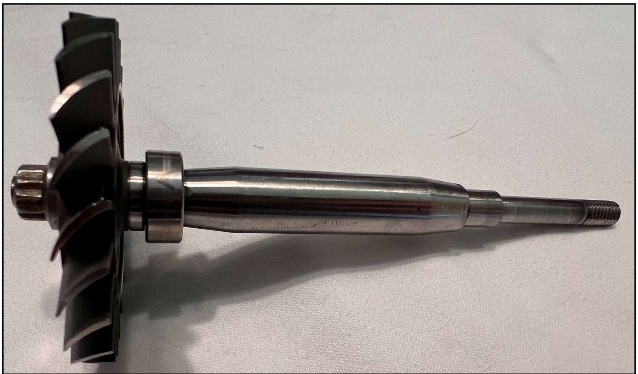
Figure 7: Completed turbine assembly
