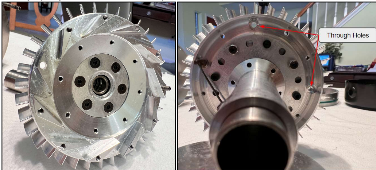
Figure 9: Through holes for fuel/oil lines of combustion chamber (right).
