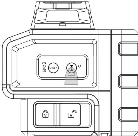
When you open pulse mode, you can use a laser receiver(not included) to carry out leveling at long distances or when the laser beams are not visible.
