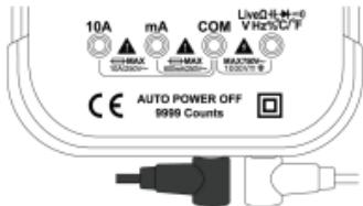
Insert the red probe into 'LiveΩHzC/F' jack and the black probe into the 'COM' jack.
